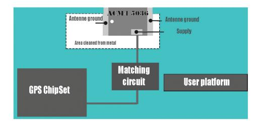
Better to move it to the top edge of PCB. As the impedance of PCB at the top edge is smaller than in long side edge, a narrower bandwidth and lower performance will be resulted than in long side of PCB.
